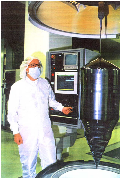
Figure 4: A silicon 'boule' is a single crystal with no lattice defects.
